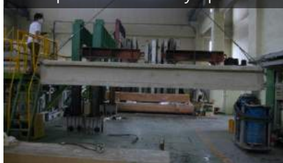
H-shape steel test body : pre-test
